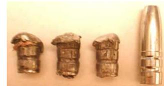
The Lyman 33889 HP, as-cast, and recovered after being expansion tested at 1600 fps.
