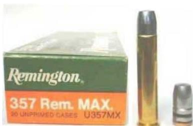
The Lyman 358156 HP is too fragile for the velocities possible with the .357 Maximum, and fragments completely at 1650 fps.
