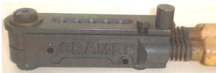
A Cramer 5 cavity .38 wadcutter mould.
