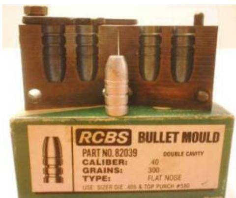
RCBS mould .40 caliber.
