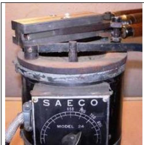
Heating an aluminum mould sprue plate down
