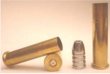
The Gould bullet (Ideal 457122), a 330 grain cast HP for the .45-70.
