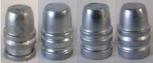
Elmer Keith's original design for the .45 Colt was the Ideal 454424 (on the left, flat-bottomed grease groove). Later, Lyman modified Keith's design to include a rounded grease groove (on right). Later on, Lyman modified this design and re-numbered it as the 452424, which has also been produced in both a flat-bottomed grease groove and rounded grease groove.
