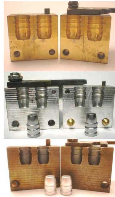
Bullet moulds can be made out of many materials. Popular materials include brass (Applegate 45 315 WFN mould, top), aluminum (Mountain Molds .40 caliber 200 grain Keith-style SWC, middle), and various ferrous alloys (RCBS 40 180 Cowboy mould, bottom).
