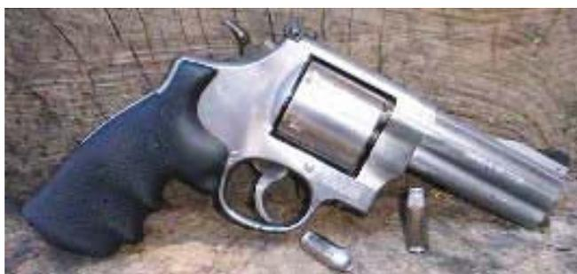
S&W 610 makes a good bowling pin gun when loaded with the Lee 175 grain truncated cone.
