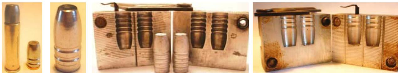
A few representative examples of LBT cast bullet designs (the .357 180 FN loaded into .357 Magnum, the LBT .357 200 grain LFN-GC, the LBT .417 305 grain LFN, the LBT .432 320 grain WLN).
