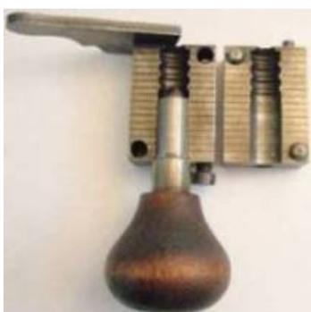
Classic wadcutter bullet moulds: the Ideal 358395 hollow-based wadcutter.
