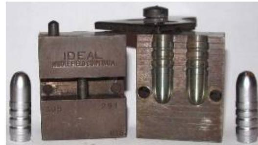
An example of an Ideal 2-cavity mould (308291).
