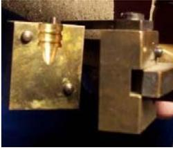
Belding & Mull made many of their moulds out of nickel. This one (for the Himmelwright wadcutter (left)) appears to be made out of brass. Yankee moulds were commonly machined out of bronze (like this 452423 mould (right)).
