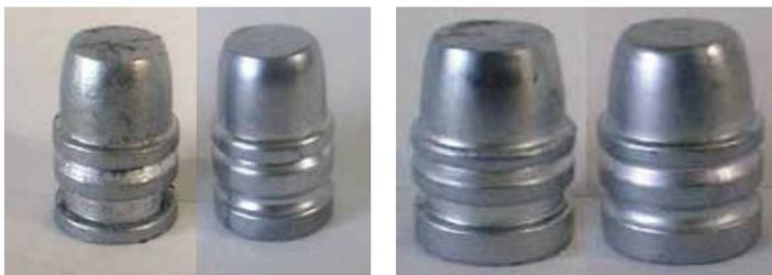
The original Ideal 454424 (left, with "square-cut" grease groove) alongside the later Lyman 454424 with a rounded grease groove. Later Lyman would re-number this to 452424, and at different times has offered that design with both flat and round grease grooves (right hand photo).
