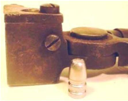
Ideal single-cavity 3118 mould for the .32-20 (integral handles).
