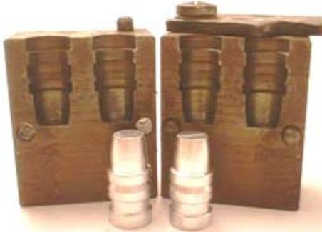
The Keith SWC (Lyman 358429) is an accurate long range revolver bullet.
