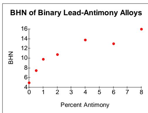
squishy plastic lead phase that's in between the hard antimony crystals. These alloys tend to be brittle because the plastic (squishy) lead phase gets its hardness from the reinforcing hard antimony rods. As the matrix gets deformed the brittle antimony rods shear off and the soft metal fails. In the case of the lead-tin alloys, the tin is more uniformly distributed through out the matrix, making the matrix itself harder, so plastic deformation of the
