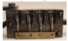
the metal's pores. After everything got burned out and the mould started producing "keepers", I recycled the rejects and the sprue's and started casting in earnest. I was recycling my sprue's as I went along, and 17 minutes later, the lead pot ran
