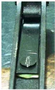
Note yellow plastic shim under the trigger spring
