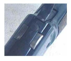
Next, metal was removed off the top of the "plug" until it was down close to same height as the top surface of the breech bolt. It was then polished, re-blued, and reinstalled.
