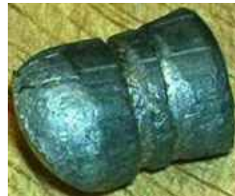
Note the rifling engraved full length of the bullet
